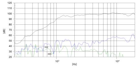
Note: On axis frequency response measured in anechoic chamber, 1W @ 1m
